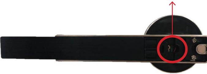
Open the cover of the back panel handle. Long press the "Reset" button for 5 seconds, and the initialization is complete
